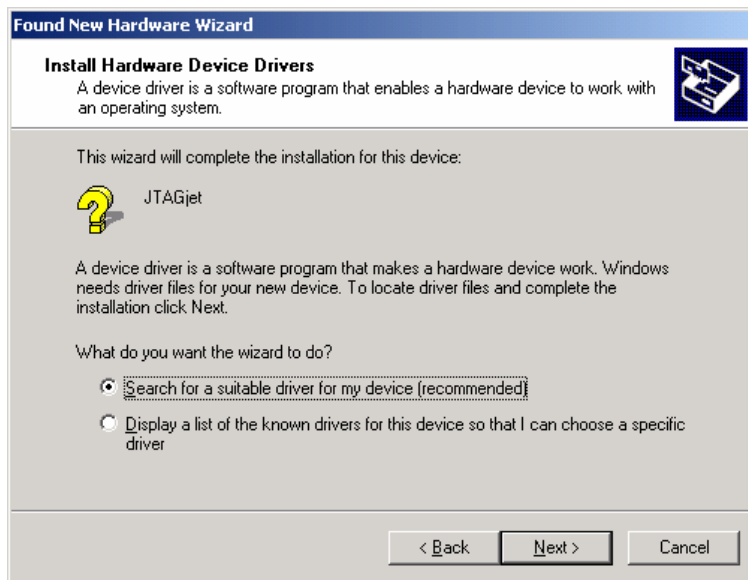
FIGURE 9 Installing the JTAGjet emulator under Windows 2000.
