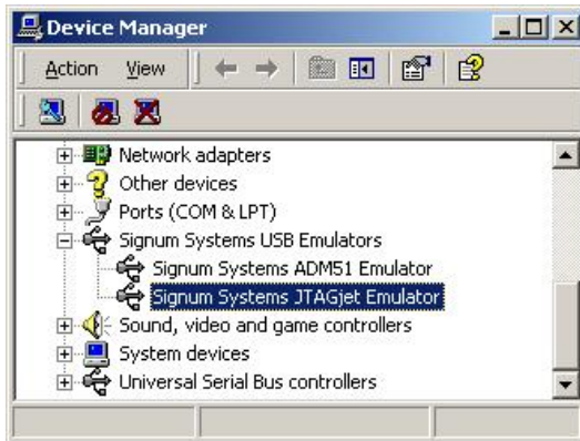
FIGURE 10 Properly installed JTAGjet and emulator listed in Device Manager.
