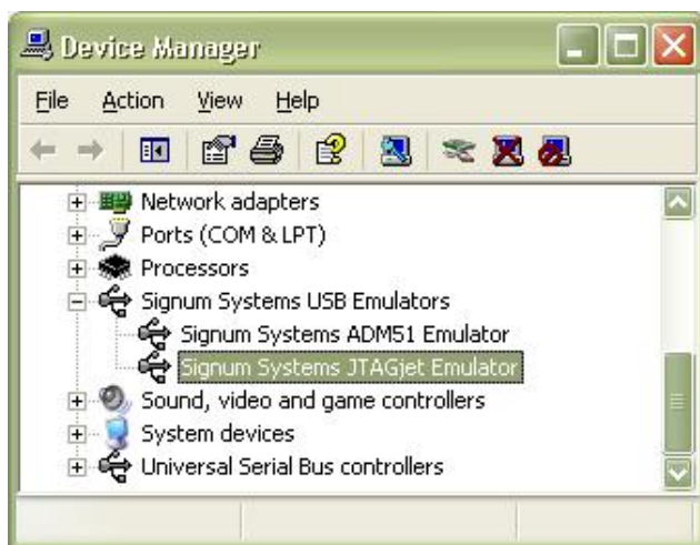
FIGURE 8 Properly installed JTAGjet emulator listed in Device Manager.
