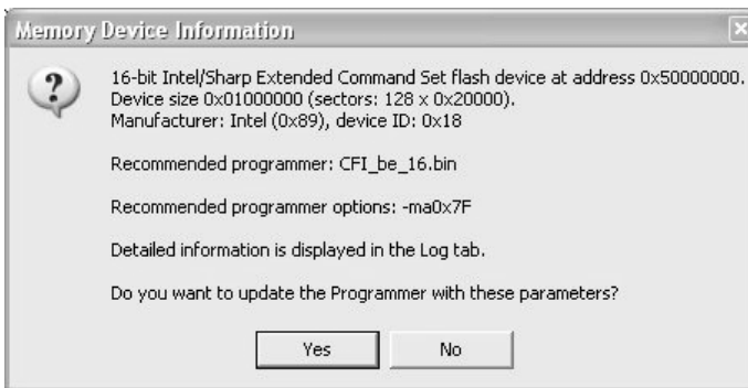
FIGURE 3 Flash query using the Query Device button. The results can be used to configure the programmer automatically.
